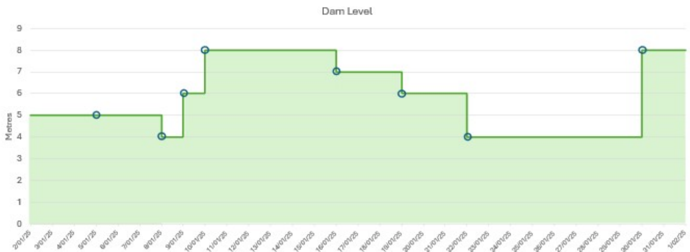
Figure 11.25. Time weighted average works well where there are missing samples
